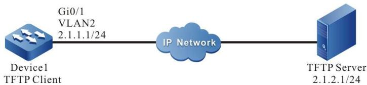
Figure 4–6 Network Topology in Which a Device Acts as a TFTP Client
