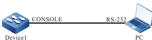
Figure 2-1 Connection for Login via the Console Port
