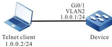
Figure 91 Network Topology for Configuring Local Authentication for Telnet User Login
