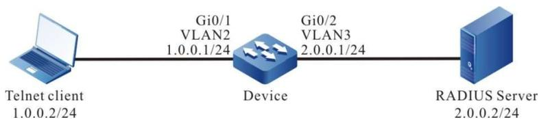
Figure 91 Network Topology for Configuring RADIUS Authentication for Telnet User Level Switch
