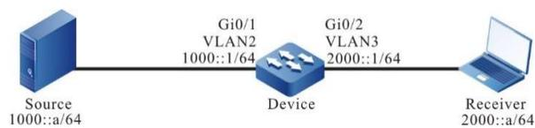
Figure 72-2 Network Topology for Configuring MLD Static Group Joining
