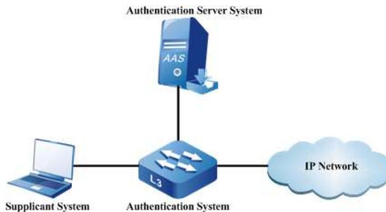
Figure 92 802.1X System Structure
