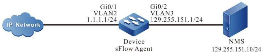
Figure 120-120 Network Topology for Configuring Basic Functions of sFlow
