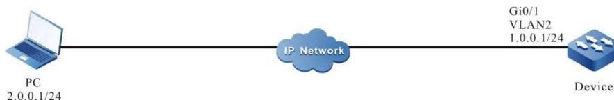
Figure 2-12 Network Topology for Configuring a Local Device to Log in to a Remote Device via SSH Public Key Authentication
