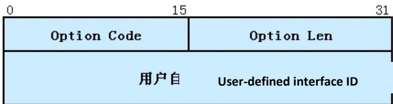
Figure 88 Extended Fill Format of Interface ID
