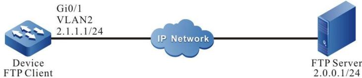
Figure4–1 Network Topology for Configuring a Device as an FTP Client
