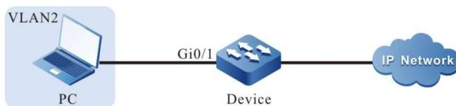
Figure 35 Network Topology for Combination of Error-disable and Storm Suppression
