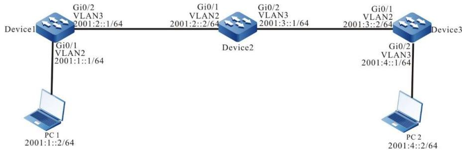
Figure 52 Network Topology for Configuring Basic Functions of IPv6 Static Route
