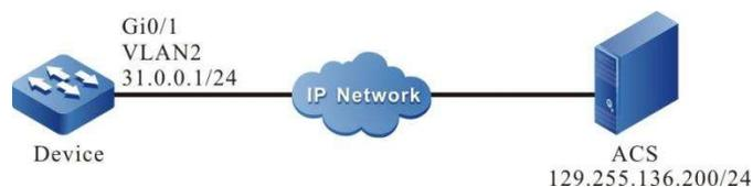
Figure 117-117 Network Topology for Configuring the CWMP Authentication Function
