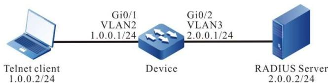
Figure 911 Network Topology for Configuring RADIUS Authentication, Authorization and Accounting for Telnet User Login
