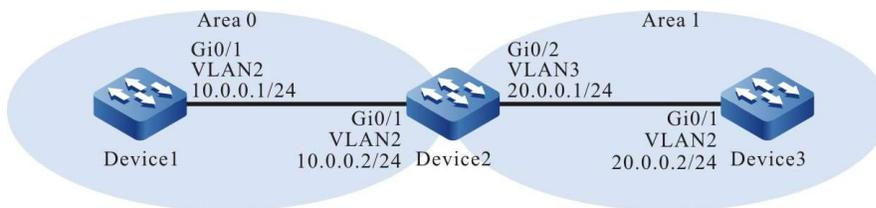
Figure 55-2 Network Topology for Configuring OSPF Authentication
