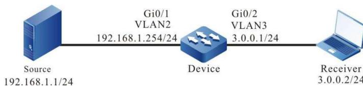
Figure 68-3 Network Topology for Configuring IGMP Static Group Joining
