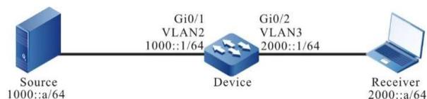
Figure 72-4 Network Topology for Configuring MLD Multicast Group Filtering
