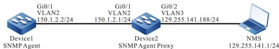
Figure 11-12 Network Topology for Configuring SNMP v3 Agent Forwarding
