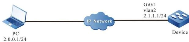
Figure4–7 Network Topology for Configuring a Device as an SFTP Client
