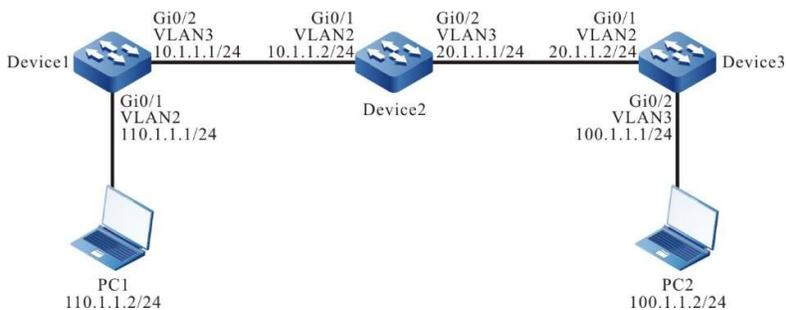
Figure 51 Network Topology for Configuring Basic Functions of Static Route
