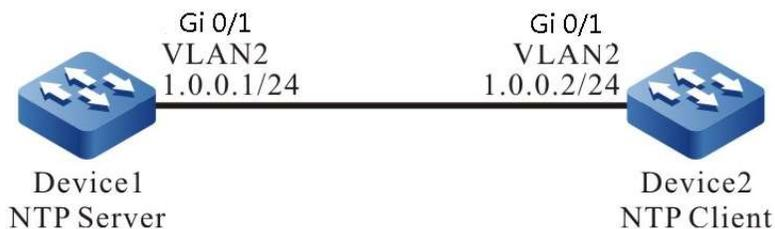
Figure 114-114 Network Topology for Configuring NTP Server and Client with MD5 Authentication
