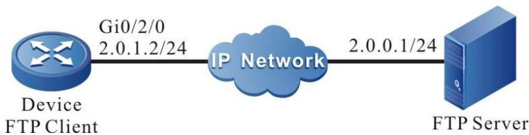
Figure 10-2 Network Topology for Upgrading of All Software Versions
