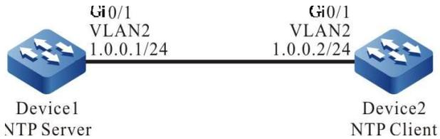
Figure 1-2 Network Topology for Configuring NTP Server and Client
