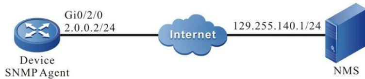
Figure 7-8 Network Topology for Configuring SNMP v3 Trap Advertisements
