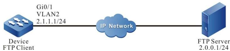
Figure 4–9 Network Topology for Configuring a Device as an FTPS Client
