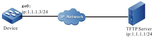
Figure 11-1 Configuring the bootloader to Boot the Image Program via the Network
