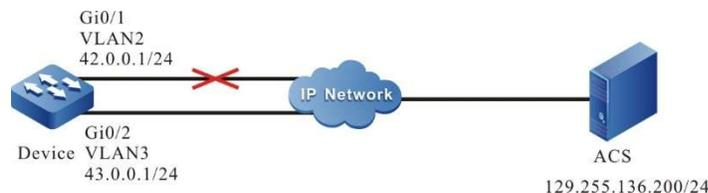
Figure 117-117 Network Topology for Configuring CWMP Link Backup
