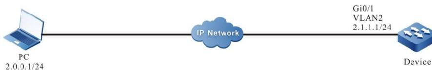
Figure 2-11 Network Topology for Configuring the Device as an SFTP Server
