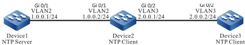
Figure 3-4 Network Topology for Configuring NTP Server and Multi-Level Client
