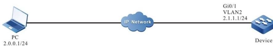
Figure 2-10 Network Topology for Configuring the Device as an SFTP Client
