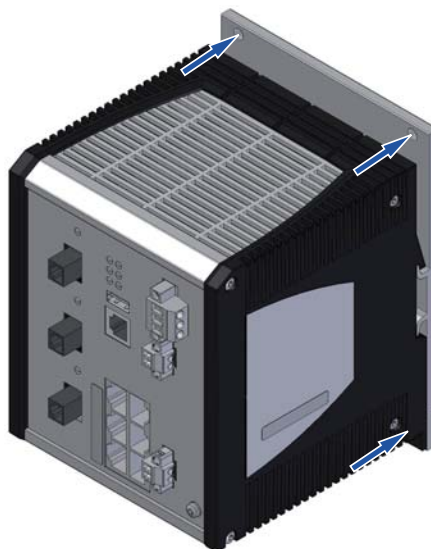
Fig. 2: Snap the device (here: RSR20/RSR30) onto the RSR wall mounting plate, screw it tightly onto the wall with 4 screws
