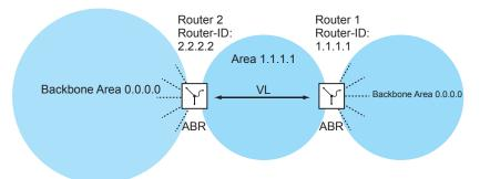
Figure 111: Expanding the backbone area using a virtual link (VL)
