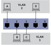
Figure 28: Example of a simple port-based VLAN
