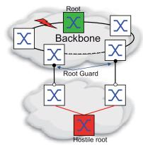
When a *Designated port* receives an STP-BPDU with better path information to the *Root bridge*, the device discards the STP-BPDU and sets the transmission state of the port to *discarding* instead of root.
