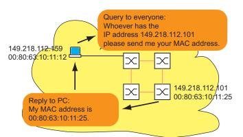
Figure 88: ARP request and reply
