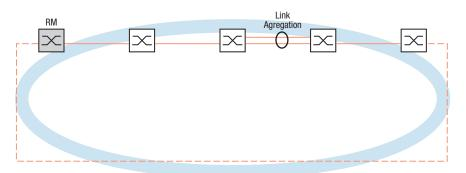
Figure 36: Link Aggregation over a single link of an MRP Ring.
