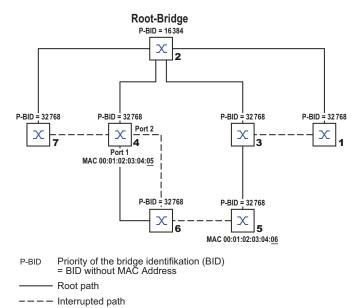
Figure 58: Example of manipulating the tree structure
