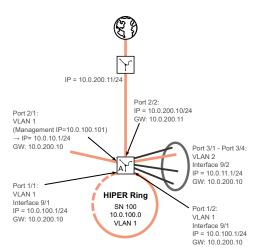
Figure 119: IP parameters for Layer 3 device A
