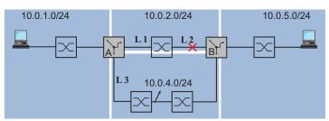
Figure 123: Example of static route tracking
