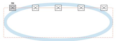
Figure 34: Redundant ring structure RM = Ring Manager — main line --- redundant line
