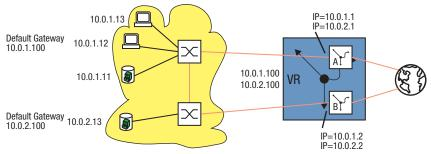
Figure 104: Virtual router with multinetting
