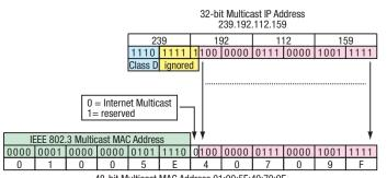
48-bit Multicast MAC Address 01:00:5E:40:70:9F Figure 116: Conversion of the IP address to the MAC address
