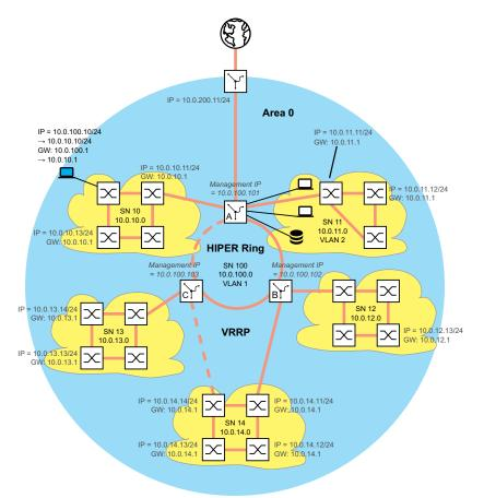
Figure 118: Network plan with management IP addresses
