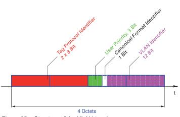
Figure 25: Structure of the VLAN tagging
