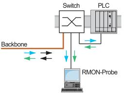
Figure 126: Application example of a port-mirroring setup
