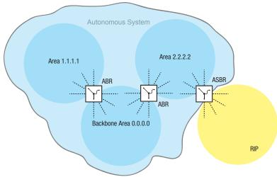
Figure 108: Autonomous System
