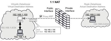
Figure 96: How the 1:1 NAT function works
