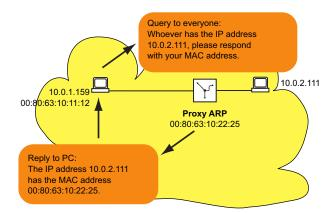
Figure 90: Proxy ARP function
