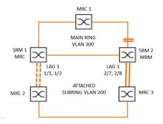
Figure 68: Sub Ring with Link Aggregation
