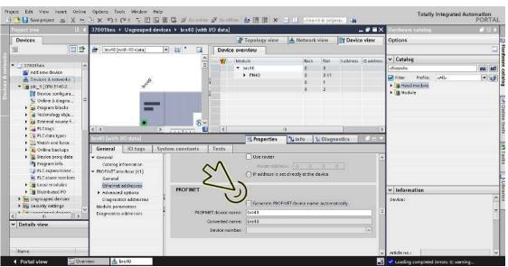
□ In the *PROFINET* frame, unmark the *Generate PROFINET* device name automatically checkbox.
