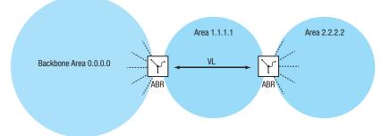
Figure 110: Linking a remote area to the backbone area using a virtual link (VL)
