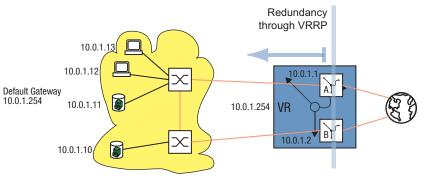
Figure 98: Illustration of the virtual router
