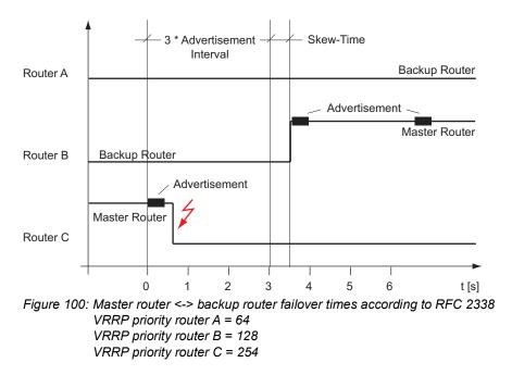
To be able to achieve faster failover times, Hirschmann developed HiVRRP which shortens the cycle for sending the IP Multicast message to as little as 0.1 seconds. You thus achieve failover times that are up to 10 times faster than VRRP.
