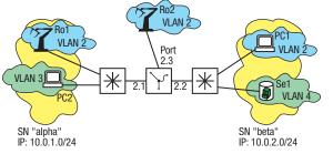
Figure 114: Application example of a protocol-based VLAN
