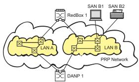
Figure 41: Parallel Redundancy Protocol Network
