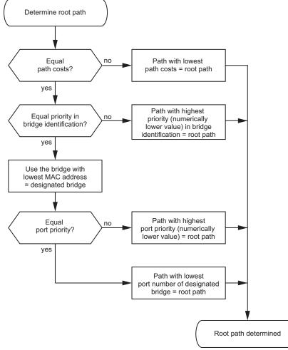
Figure 55: Flow diagram for specifying the root path
