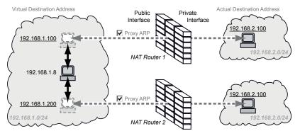
Figure 97: Connect identical production cells with the host computer (application example)
