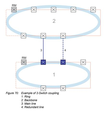
In a 2-Switch coupling (see figure 70), the 2 devices have specific roles:
