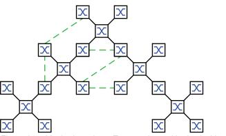
Figure 31: Meshed topology: Tree topology with physical loops
