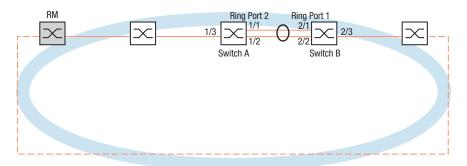
Figure 39: Application example of an MRP over LAG setup
