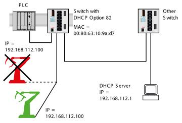
Figure 128: Application example of using Option 82
