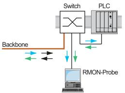
*Figure 87: Application example of a port-mirroring setup*
