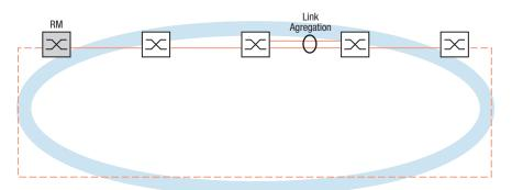
Figure 35: Link Aggregation over a single link of an MRP Ring.
