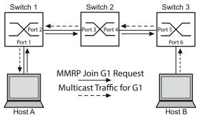
Figure 100: MMRP Network for MAC address Registration
