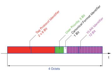
Figure 24: Structure of the VLAN tagging
