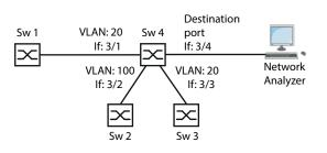
Figure 88: Application example of a VLAN mirroring setup
