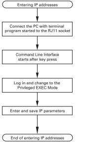
Figure 14: Flow chart for entering IP addresses
