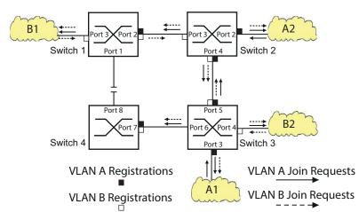
Figure 101: MVRP Example Network for VLAN Registration
