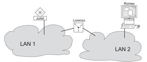
Figure 11: The management agent is separated from its network management station by a router
