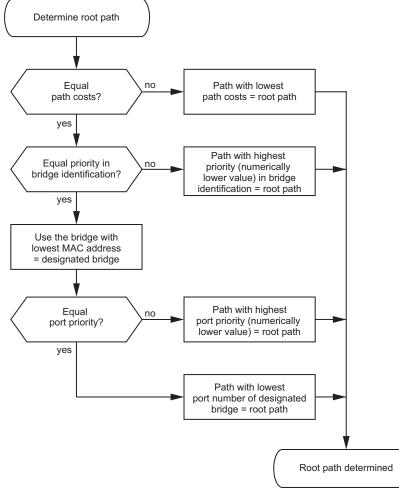
Figure 54: Flow diagram for specifying the root path
