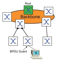
Ports connected to an end device do not normally receive any STP-BPDUs. If an attacker still attempts to feed in STP-BPDUs on this port, then the device deactivates the port.
