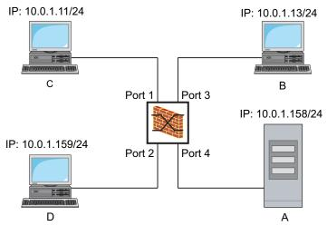
Figure 22: Application example of an IPACL
