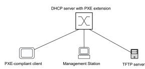
Figure 98: Simple structure of a Preboot eXecution Environment (PXE) setup
