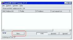
Figure 125: Adding static addresses
