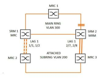
Figure 67: Sub Ring with Link Aggregation
