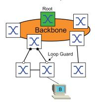
If the port does not receive any more STP-BPDUs, then this protection function helps prevent the transmission status of a port from unintentionally being changed to *forwarding*. If this situation occurs, then the device designates the loop status of the port as inconsistent, but does not forward any data packets.
