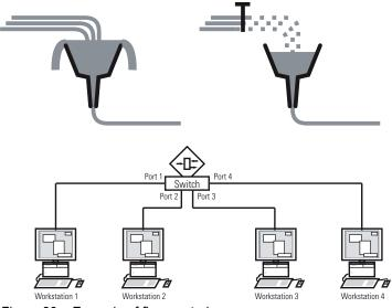
Figure 26: Example of flow control
