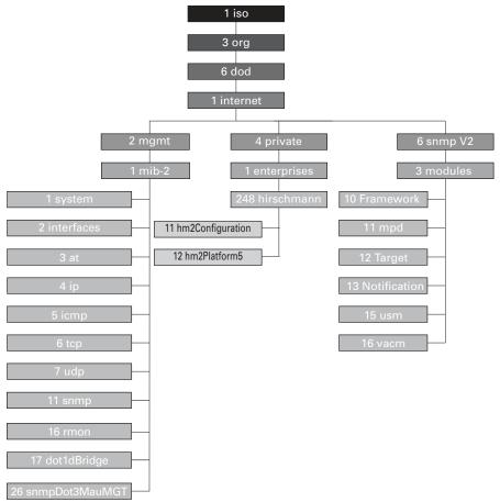
Figure 131: Tree structure of the Hirschmann MIB
