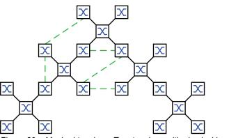
Figure 30: Meshed topology: Tree topology with physical loops
