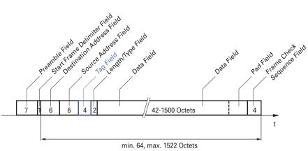
Figure 23: Ethernet data packet with tag
