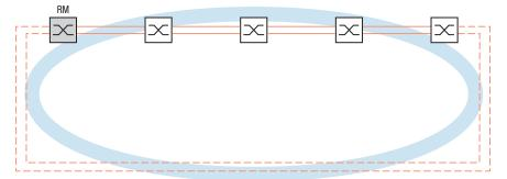
Figure 36: Link Aggregation over the entire MRP Ring.
