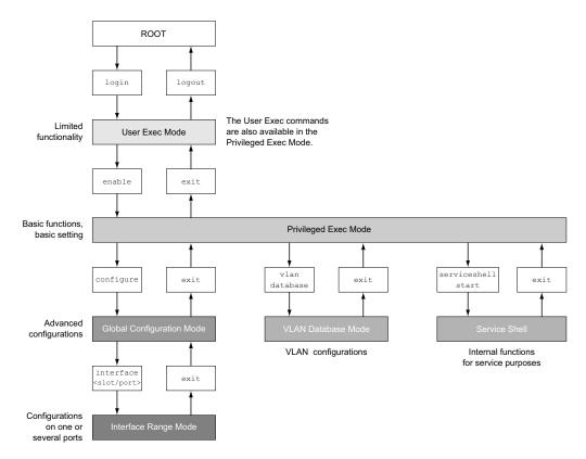
Figure 6: Structure of the Command Line Interface
