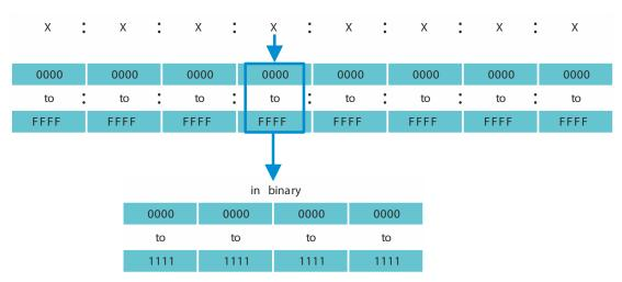
Figure 12: IPv6 address representation
