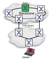
If the protection function is activated, then the device ignores *Topology Change* flags in received STP-BPDUs. This does not change the content of the MAC address table (forwarding database) of the port. However, additional information in the BPDU that changes the topology is processed by the device.
