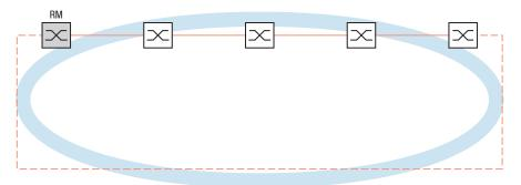
Figure 33: Redundant ring structure RM = Ring Manager — main line --- redundant line
