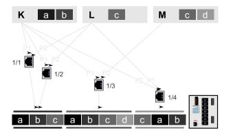
When assigning the ACLs to ports 1/1 to 1/4, the device writes the rules contained in that ACLs with the specified priority to a hardware memory area that the ports and VLANs share. The order of the rules in relation to each other is determined by the index number within the respective ACL and by the assignment priority.
