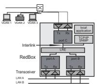
Figure 41: RedBox Transition from double to single LAN
