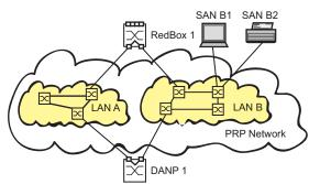
Figure 40: Parallel Redundancy Protocol Network
