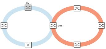
*Figure 64:* Special case: A Sub Ring Manager device manages both ends of a Sub Ring on different ports (Single Sub Ring Manger).
