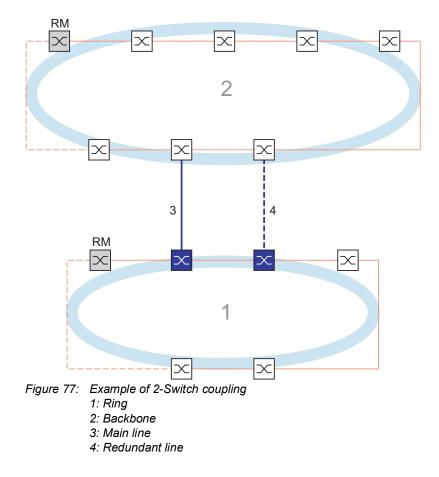
The coupling between 2 networks is performed by the main line, indicated by the solid blue line. If the main line or one of the connected devices becomes inoperable, then the redundant line, indicated by the dashed black line, takes over the network coupling. The coupling is performed by 2 devices.
