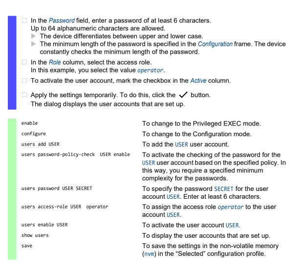
**Note:** When you are setting up a new user account in the Command Line Interface, remember to allocate the password.
