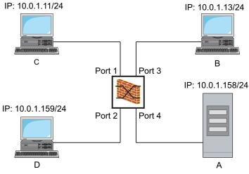
Figure 22: Application example of an IPACL
