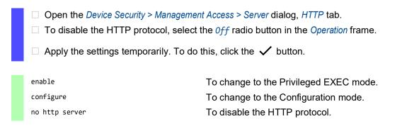
If the HTTP protocol is disabled, then you can reach the Graphical User Interface of the device only by HTTPS. In the address bar of the web browser, enter the string https://before the IP address of the device.
