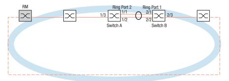
Figure 38: Application example of an MRP over LAG setup
