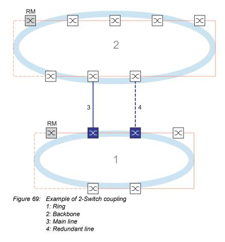
In a 2-Switch coupling (see figure 69), the 2 devices have specific roles:
