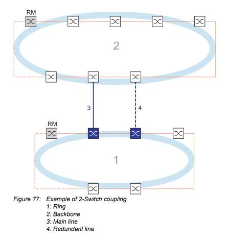
The coupling between 2 networks is performed by the main line, indicated by the solid blue line. If the main line or one of the connected devices becomes inoperable, then the redundant line, indicated by the dashed black line, takes over the network coupling. The coupling is performed by 2 devices.
