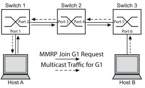
Figure 99: MMRP Network for MAC address Registration
