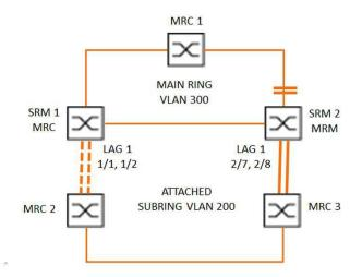
Figure 67: Sub Ring with Link Aggregation
