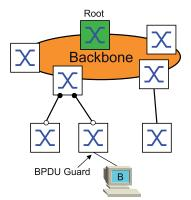
Terminal device ports do not normally receive any STP-BPDUs. If an attacker still attempts to feed in STP-BPDUs on this port, then the device deactivates the device port.
