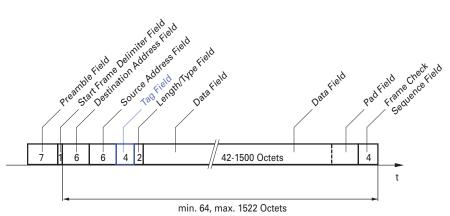
Figure 24: Ethernet data packet with tag
