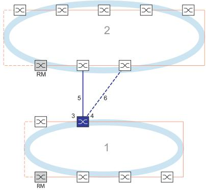
Figure 70: Example of 1-Switch coupling
