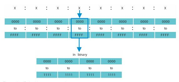
Figure 12: IPv6 address representation
