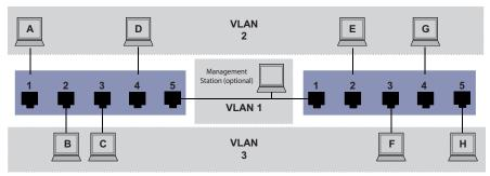
Figure 29: Example of a more complex VLAN configuration
