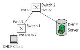
Figure 130: DHCP Layer 2 Example Network
