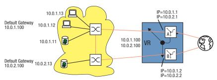
Figure 97: Virtual router with multinetting
