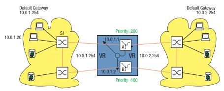
Figure 96: Virtual router with load sharing
