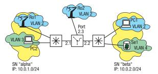
Figure 107: Application example of a protocol-based VLAN
