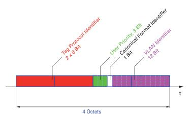
Figure 25: Structure of the VLAN tagging
