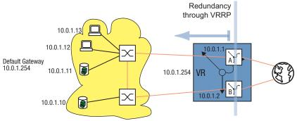
Figure 91: Illustration of the virtual router
