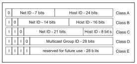
Figure 10: Bit representation of the IP address
