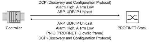
Figure 138: Communication between the Controller and the device
