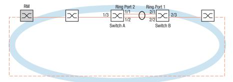
Figure 43: Application example of an MRP over LAG setup
