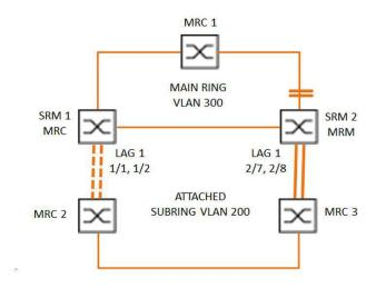
Figure 62: Sub Ring with Link Aggregation
