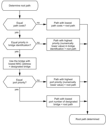
Figure 49: Flow diagram for specifying the root path
