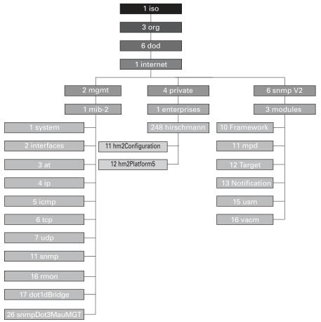
Figure 162: Tree structure of the Hirschmann MIB
