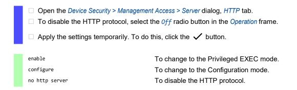
If the HTTP protocol is disabled, then you can reach the Graphical User Interface of the device only by HTTPS. In the address bar of the web browser, enter the string https:// before the IP address of the device.
