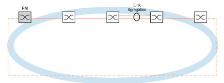
Figure 40: Link Aggregation over a single link of an MRP Ring.
