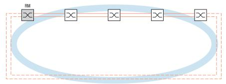
Figure 41: Link Aggregation over the entire MRP Ring.
