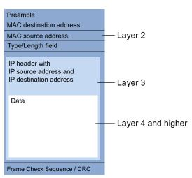
Figure 83: Structure of a data packet from the ISO/OSI reference model perspective
