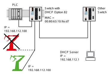
Figure 159: Application example of using Option 82
