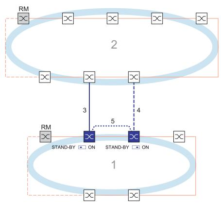
Figure 67: Example of 2-Switch coupling with control line
