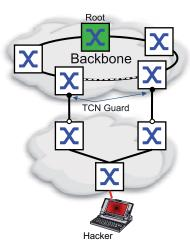
If the protection function is activated, then the device ignores *Topology Change* flags in received STP-BPDUs. This does not change the content of the MAC address table (forwarding database) of the device port. However, additional information in the BPDU that changes the topology is processed by the device.
