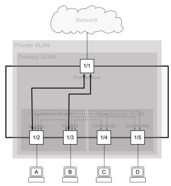
Figure 31: Communication flow of the isolated ports
