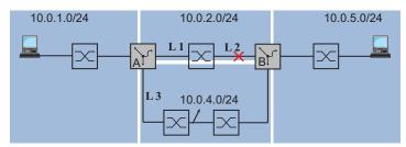
Figure 116: Example of static route tracking
