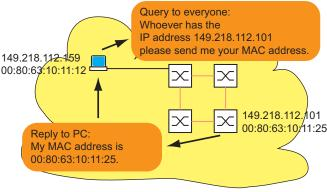
Figure 82: ARP request and reply
