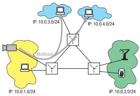
Figure 108: Example of a multicast application
