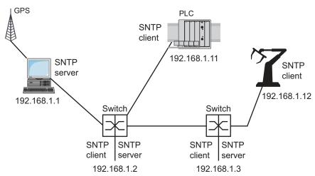
Figure 20: Example of SNTP cascade
