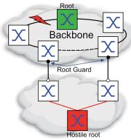
When a *Designated port* receives an STP-BPDU with better path information to the *Root bridge*, the device discards the STP-BPDU and sets the transmission state of the port to *discarding* instead of root.
