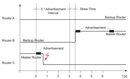
Figure 93: Master router <-> backup router failover times according to RFC 2338
