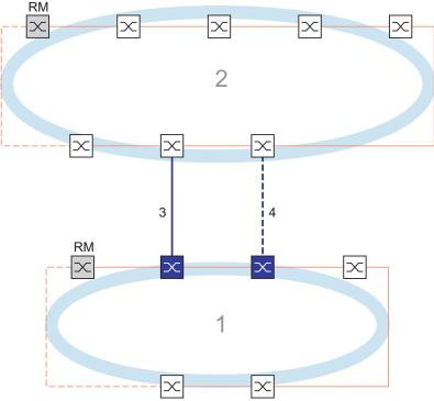
Figure 72: Example of 2-Switch coupling
