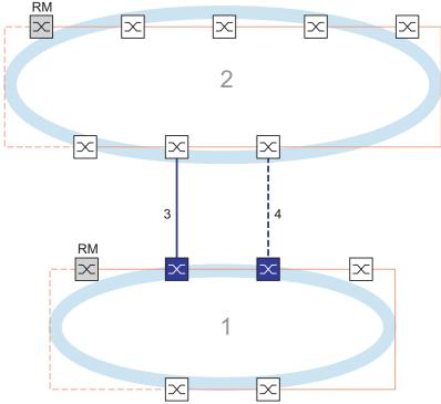
Figure 64: Example of 2-Switch coupling
