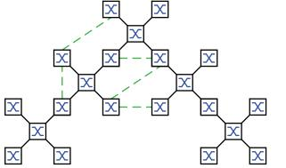
Figure 35: Meshed topology: Tree topology with physical loops
