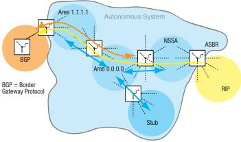
Figure 102: LSA distribution into the area types
