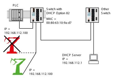
Figure 123: Application example of using Option 82
