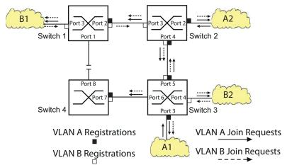
Figure 96: MVRP Example Network for VLAN Registration
