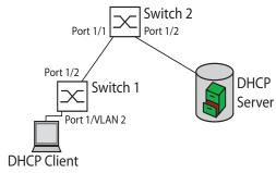
Figure 93: DHCP Layer 2 Example Network
