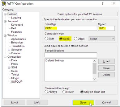
Figure 4:Serial connection using the PuTTY program
