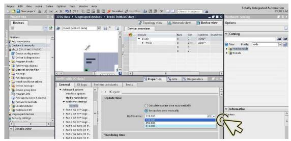
☐ In the Watchdog time frame, select the desired item from the Accepted update cycles without IO data drop-down list.
