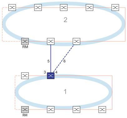
Figure 62: Example of 1-Switch coupling
