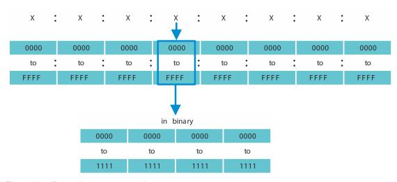
Figure 12: IPv6 address representation
