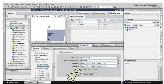
☐ Mark the *Diagnostics interrupts* checkbox to receive *MRP* ring Open/Close alarms.
