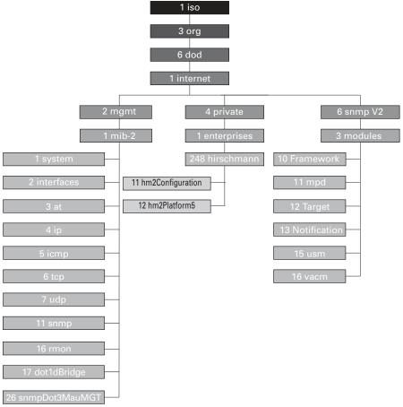
Figure 126: Tree structure of the Hirschmann MIB
