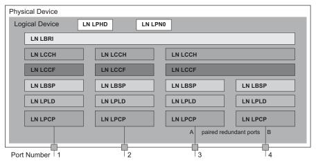
Figure 98: Bridge model based on Technical Report IEC 61850 90-4
