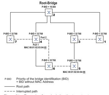
Figure 51: Example of manipulating the tree structure
