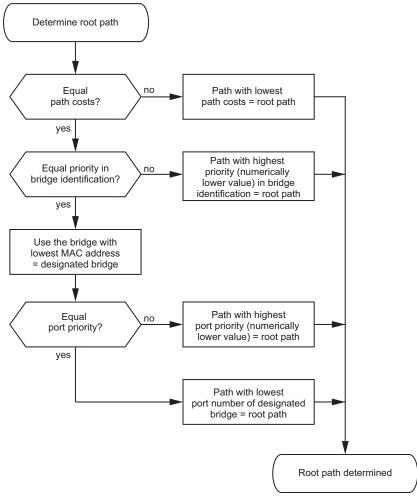
Figure 48: Flow diagram for specifying the root path
