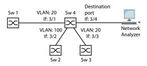
Figure 82: Application example of a VLAN mirroring setup
