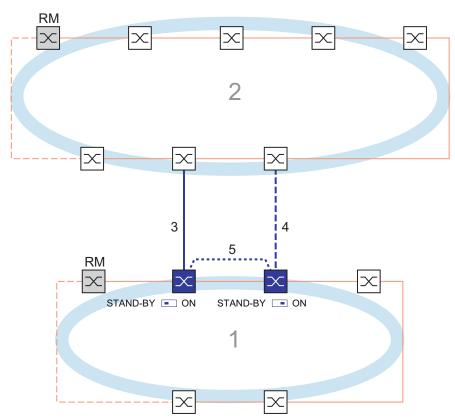
Figure 66: Example of 2-Switch coupling with control line
