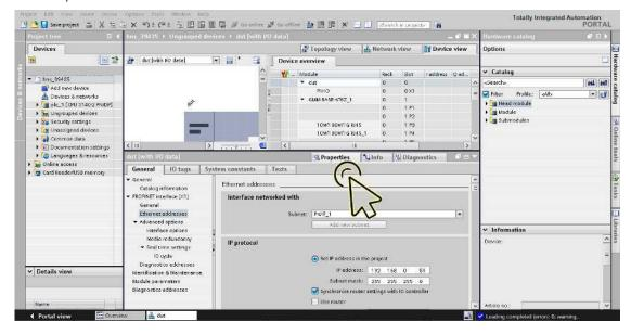
□ In the General tab, navigate to the PROFINET interface [X1] > Advanced options > Real time settings > IO cycle item.
