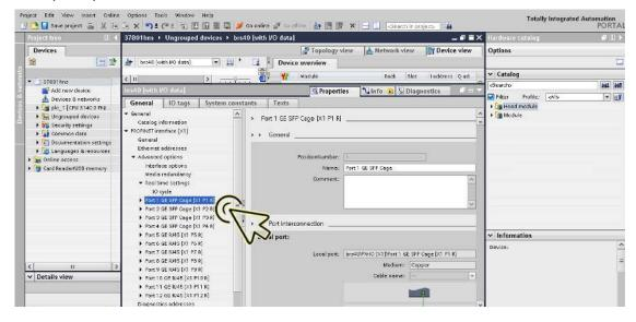
☐ In the *Port options* section, *Connection* frame, select the desired item from the *Transmission rate/duplex* drop-down list other than the *Automatic* item.
