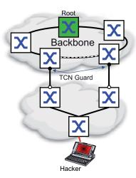
If the protection function is activated, then the device ignores *Topology Change* flags in received STP-BPDUs. This does not change the content of the MAC address table (forwarding database) of the port. However, additional information in the BPDU that changes the topology is processed by the device.
