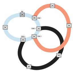
Figure 56: Example of an overlapping Sub Ring structure
