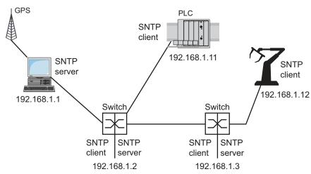
Figure 19: Example of SNTP cascade
