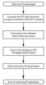
Figure 14: Flow chart for entering IP addresses
