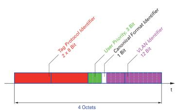
Figure 24: Structure of the VLAN tagging
