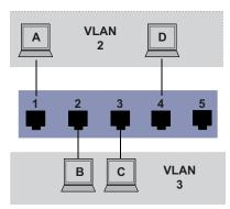
Figure 27: Example of a simple port-based VLAN
