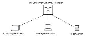
Figure 92: Simple structure of a Preboot eXecution Environment (PXE) setup
