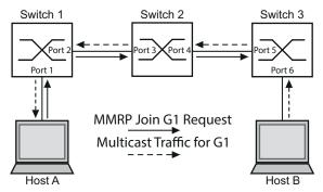
Figure 95: MMRP Network for MAC address Registration
