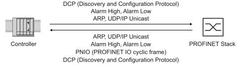
Figure 102: Communication between the Controller and the device
