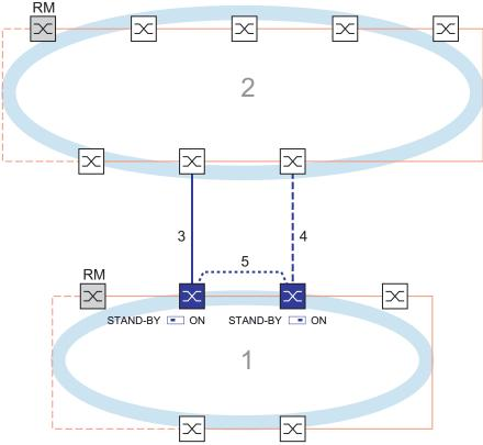
Figure 74: Example of 2-Switch coupling with control line
