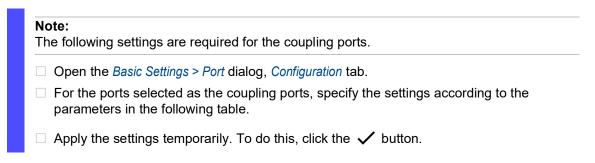
To minimize the ring recovery time in case of a link-up after a failure, set up the speed and duplex mode of the ring ports as follows:
