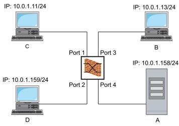
Figure 22: Application example of an IP ACL
