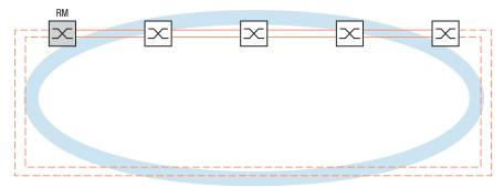
Figure 40: Link Aggregation over the entire MRP Ring.
