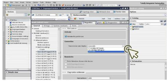
The device automatically marks the Monitor and Enable autonegotiation checkboxes.
