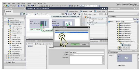
As an alternative, click the Not assigned link in the device tile, then select the required item.
