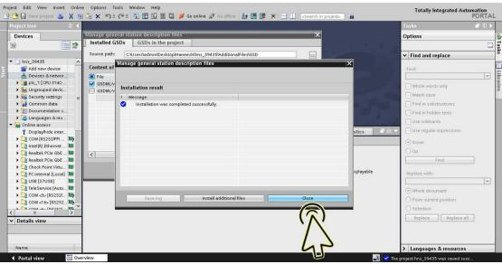
You find the new device under the items Other field devices > PROFINET IO > Network Components > Hirschmann Automation and Control GmbH.
