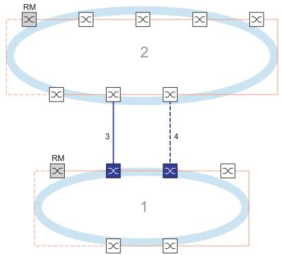
Figure 71: Example of 2-Switch coupling
