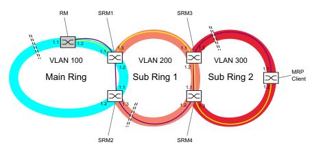
Figure 60: Example of a cascaded Sub Ring structure
