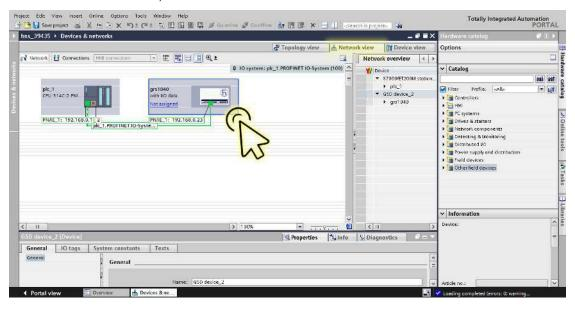
☐ Select the *Device view* tab to display the device details.
