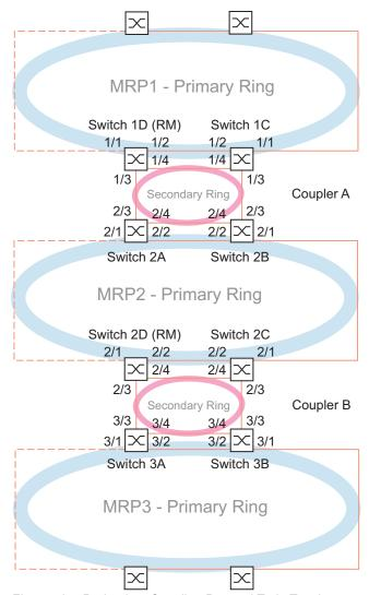
Figure 78: Redundant Coupling Protocol Train Topology:
