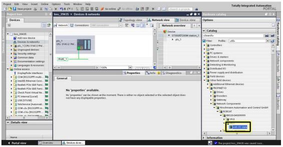
☐ Drag the selected device and drop it onto the *Network view* worksheet.
