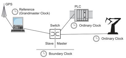
Figure 20: Position of the boundary clock in a network
