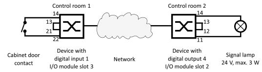
Figure 94: Mirroring an I/O signal over the network
