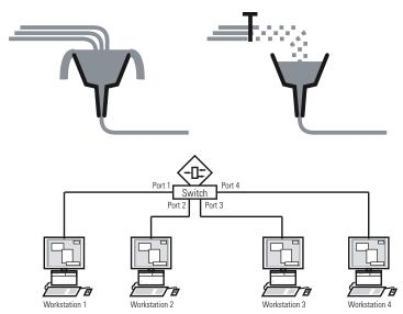
Figure 26: Example of flow control
