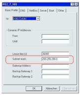
Figure 111:Netmask in the configuration profile
