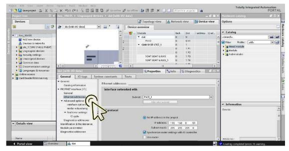
☐ In the IP protocol frame, select the Set IP address in the project radio button.
