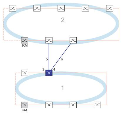
Figure 69: Example of 1-Switch coupling
