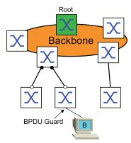
Ports connected to an end device do not normally receive any STP-BPDUs. If an attacker still attempts to feed in STP-BPDUs on this port, then the device deactivates the port.
