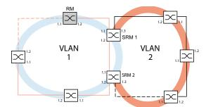
Figure 59: Example of a Sub Ring structure with VLANs orange line= Main ring members in VLAN 1 black line= Sub Ring members in VLAN 2 orange dashed line= Main ring loop open black dashed line= Sub Ring loop open SRM = Sub Ring Manager RM = Ring Manager
