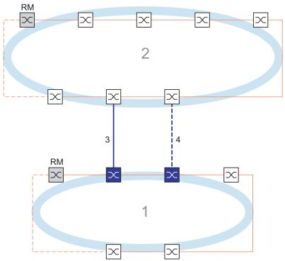
Figure 63: Example of 2-Switch coupling
