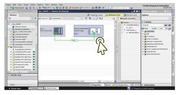
☐ Select the *Device view* tab to display the device details.
