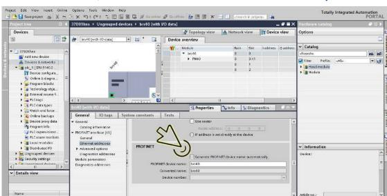
☐ In the PROFINET frame, unmark the Generate PROFINET device name automatically checkbox.
