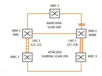
Figure 61: Sub Ring with Link Aggregation
