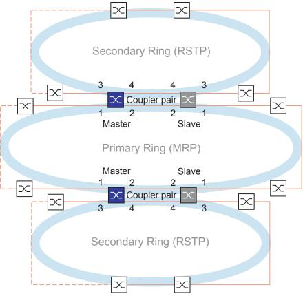
Figure 77: Example of a two-switch redundant coupling (2 coupler pairs)
