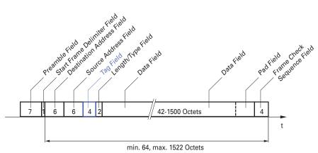
Figure 23: Ethernet data packet with tag
