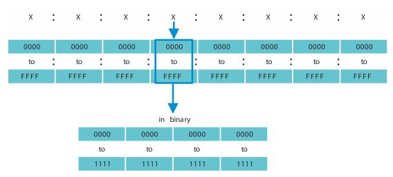
Figure 12: IPv6 address representation
