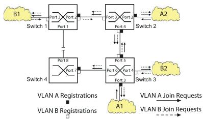
Figure 94: MVRP Example Network for VLAN Registration
