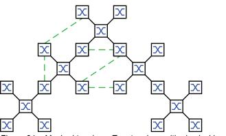
Figure 34: Meshed topology: Tree topology with physical loops
