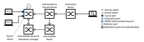
Figure 87: Example of a simple ring topology based on an existing redundant ring (with shared links)
