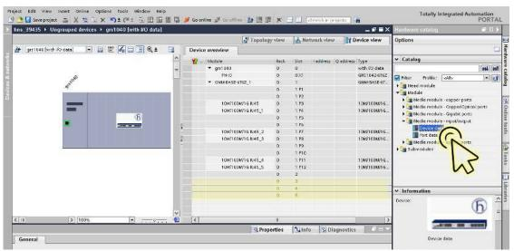
In the Device view tab, the slot which is logically connected to the device is highlighted.
