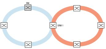
*Figure 58:* Special case: A Sub Ring Manager device manages both ends of a Sub Ring on different ports (Single Sub Ring Manger).
