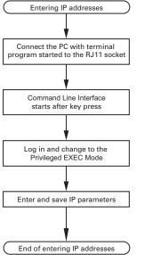
Figure 14: Flow chart for entering IP addresses
