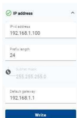
Figure 8: Assigning IP parameters using the Provize Explorer application
