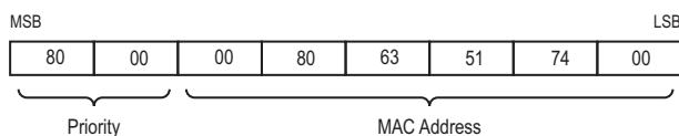
Figure 33: Bridge Identifier, Example (interpretation according to IEEE 802.1D-1998, values in hexadecimal notation)
