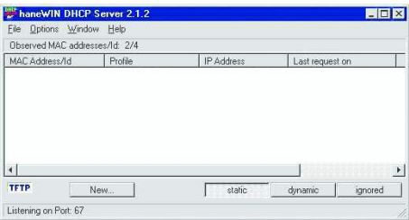
Figure 109: Start window of the haneWIN DHCP Server program
