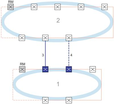
Figure 72: Example of 2-Switch coupling
