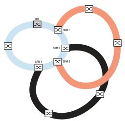
Figure 57: Example of an overlapping Sub Ring structure
