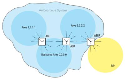
Figure 101: Autonomous System
