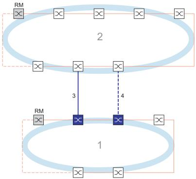
Figure 64: Example of 2-Switch coupling
