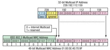
Figure 109: Conversion of the IP address to the MAC address
