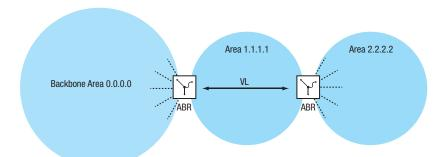
Figure 103: Linking a remote area to the backbone area using a virtual link (VL)
