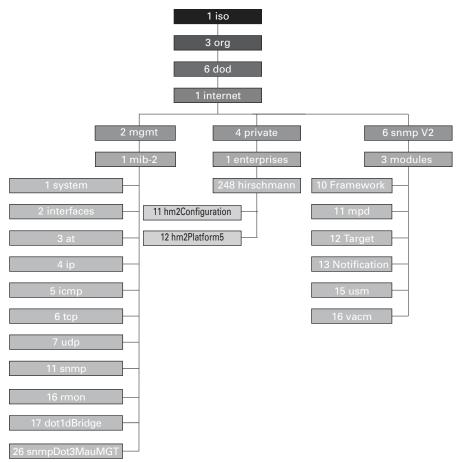
Figure 161: Tree structure of the Hirschmann MIB
