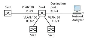
Figure 120: Application example of a VLAN mirroring setup
