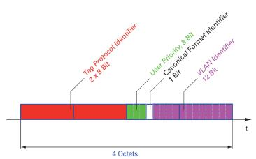
Figure 25: Structure of the VLAN tagging
