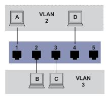
Figure 28: Example of a simple port-based VLAN
