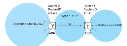
Figure 104: Expanding the backbone area using a virtual link (VL)
