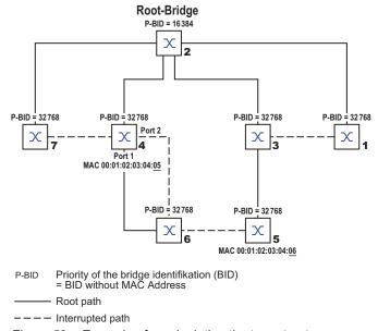
Figure 52: Example of manipulating the tree structure
