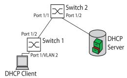
Figure 130: DHCP Layer 2 Example Network
