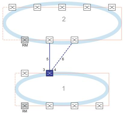
Figure 63: Example of 1-Switch coupling
