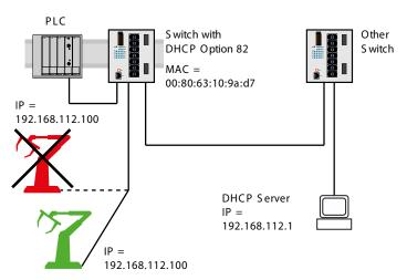
Figure 158: Application example of using Option 82
