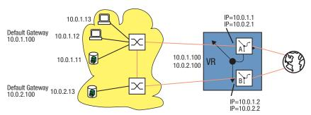
Figure 97: Virtual router with multinetting
