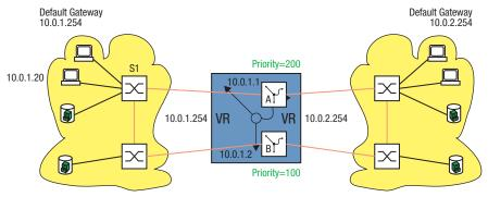
Figure 96: Virtual router with load sharing
