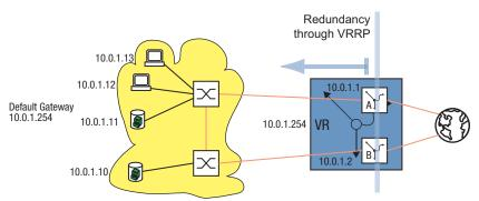
Figure 91: Illustration of the virtual router
