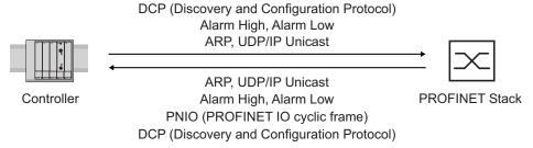
Figure 137: Communication between the Controller and the device
