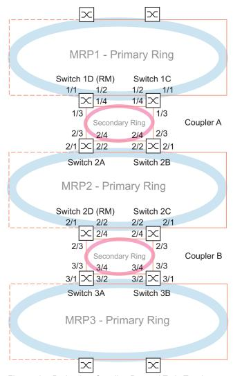
Figure 79: Redundant Coupling Protocol Train Topology:
