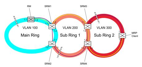
Figure 61: Example of a cascaded Sub Ring structure
