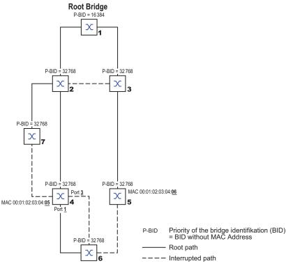
Figure 50: Example of a network plan for determining the root path
