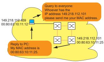
Figure 82: ARP request and reply
