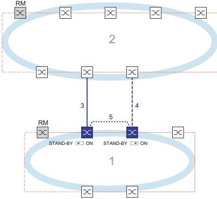
Figure 75: Example of 2-Switch coupling with control line
