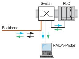
Figure 119: Application example of a port-mirroring setup
