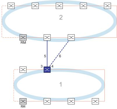
Figure 70: Example of 1-Switch coupling
