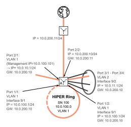
Figure 112: IP parameters for Layer 3 device A
