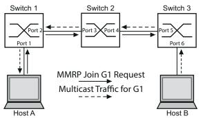
Figure 131: MMRP Network for MAC address Registration
