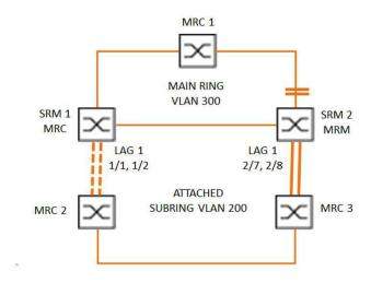
Figure 62: Sub Ring with Link Aggregation
