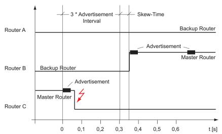
Figure 94: Master router <-> backup router failover times according to HiVRRP VRRP priority router A = 64
