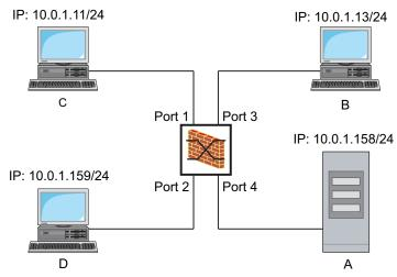
Figure 23: Application example of an IPACL
