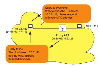
Figure 84: Proxy ARP function
