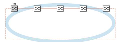
Figure 38: Redundant ring structure RM = Ring Manager —— main line - - - redundant line
