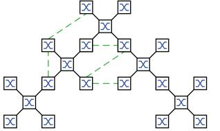
Figure 35: Meshed topology: Tree topology with physical loops
