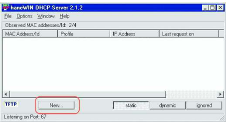
Figure 70: Adding static addresses
