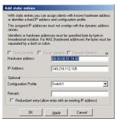
Figure 153:Entries for static addresses
