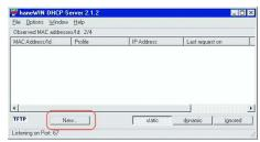
Figure 157: Adding static addresses
