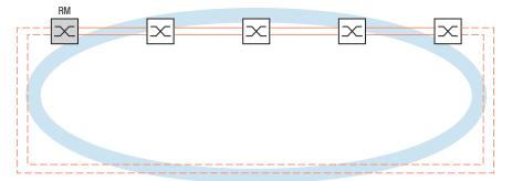
Figure 41: Link Aggregation over the entire MRP Ring.
