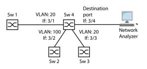
Figure 120: Application example of a VLAN mirroring setup
