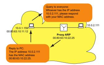
Figure 84: Proxy ARP function
