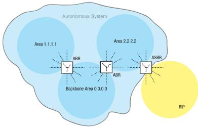
Figure 101: Autonomous System
