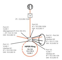
Figure 112: IP parameters for Layer 3 device A
