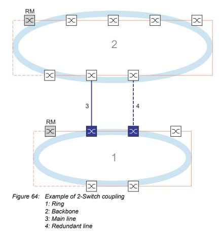
In a 2-Switch coupling (see figure 64), the 2 devices have specific roles:
