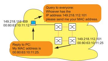
Figure 82: ARP request and reply
