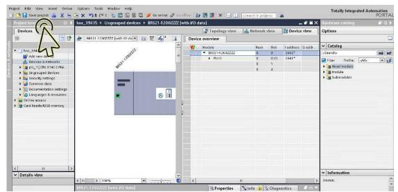
**Note:** *PROFINET* monitors the topology configuration. If you connect the port of the Hirschmann device to a different port of the partner device, then the Hirschmann device generates an alarm with the error message Wrong partner port.
