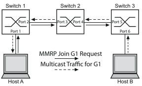
Figure 131: MMRP Network for MAC address Registration
