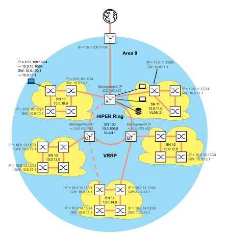
Figure 111: Network plan with management IP addresses
