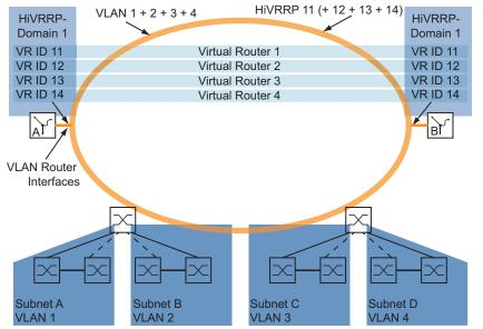
Figure 95: Example of how a HiVRRP domain is used
