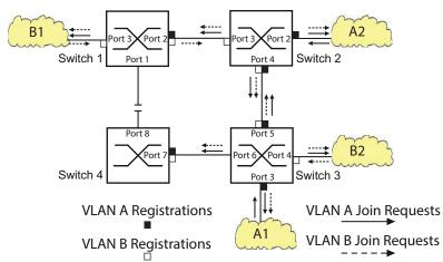
Figure 132: MVRP Example Network for VLAN Registration
