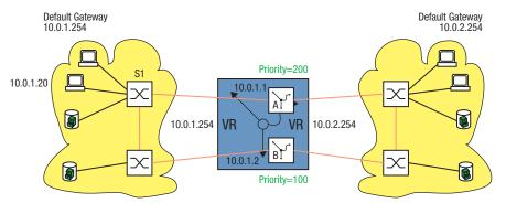
Figure 96: Virtual router with load sharing
