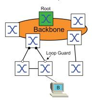
If the port does not receive any more STP-BPDUs, then this protection function helps prevent the transmission status of a port from unintentionally being changed to *forwarding*. If this situation occurs, then the device designates the loop status of the port as inconsistent, but does not forward any data packets.
