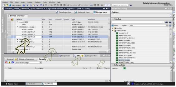
Drag the selected SFP submodule, and drop it onto the highlighted slot in the *Device view* tab.
