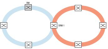
Figure 59: Special case: A Sub Ring Manager device manages both ends of a Sub Ring on different ports (Single Sub Ring Manger).
