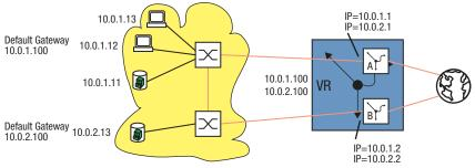
Figure 97: Virtual router with multinetting
