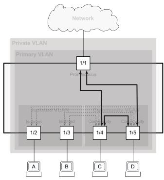
Figure 32: Communication flow of the community ports
