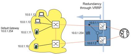
Figure 91: Illustration of the virtual router
