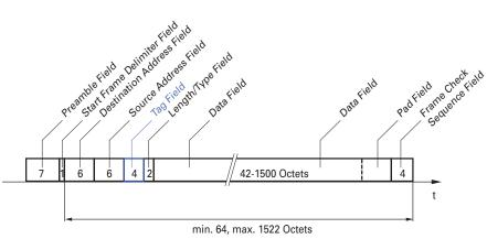
Figure 24: Ethernet data packet with tag
