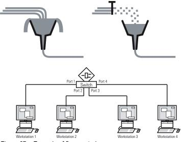
Figure 27: Example of flow control
