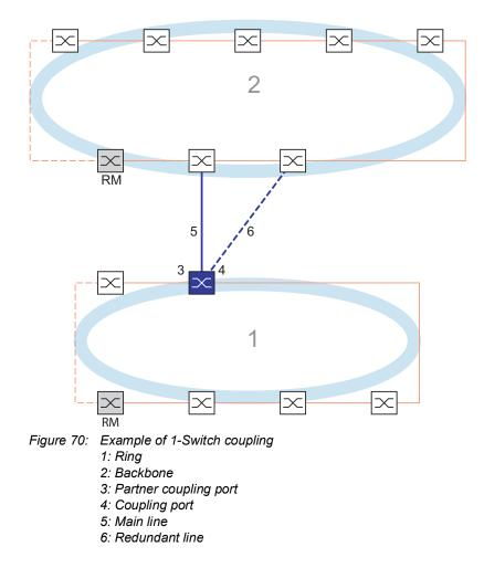
The main line, indicated by the solid blue line, which is connected to the partner coupling port provides coupling between the two networks in the normal mode of operation. If the main line is inoperable, then the redundant line, indicated by the dashed blue line, which is connected to the coupling port takes over the ring/network coupling. **One** switch performs the coupling switch-over.
