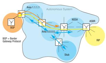
Figure 102: LSA distribution into the area types
