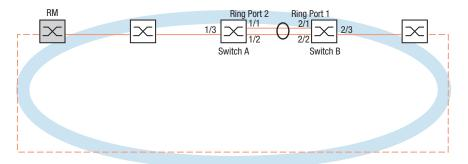
Figure 42: Application example of an MRP over LAG setup
