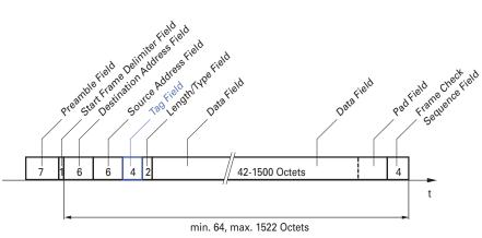
Figure 23: Ethernet data packet with tag
