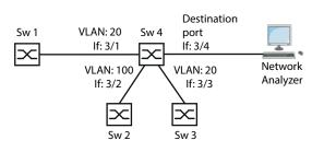
Figure 82: Application example of a VLAN mirroring setup
