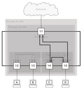
Figure 31: Communication flow of the community ports
