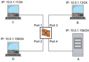
Figure 22: Application example of an IPACL
