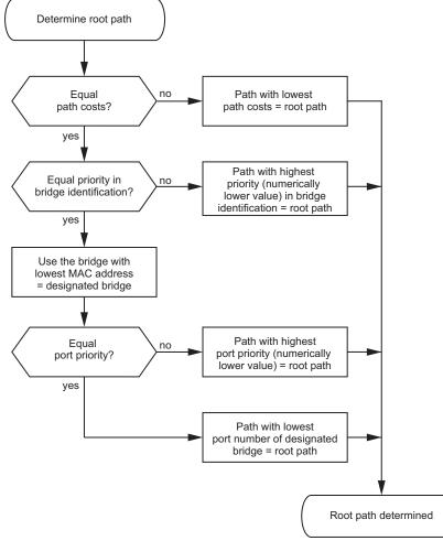
Figure 48: Flow diagram for specifying the root path
