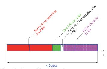
Figure 24: Structure of the VLAN tagging
