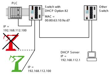
Figure 121: Application example of using Option 82
