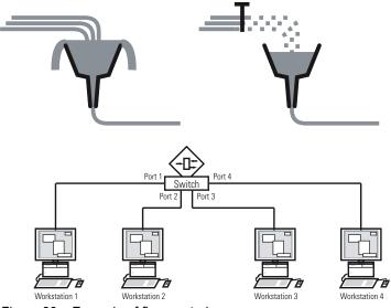
Figure 26: Example of flow control
