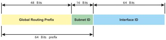
Figure 13: IPv6 Global Unicast address general format
