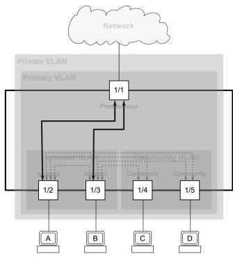
Figure 30: Communication flow of the isolated ports
