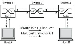
Figure 93: MMRP Network for MAC address Registration
