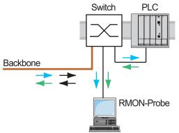
Figure 81: Application example of a port-mirroring setup
