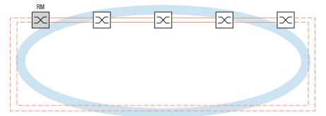
Figure 40: Link Aggregation over the entire MRP Ring.
