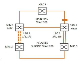
Figure 61: Sub Ring with Link Aggregation
