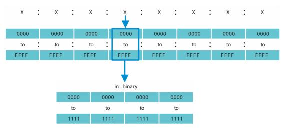
Figure 12: IPv6 address representation
