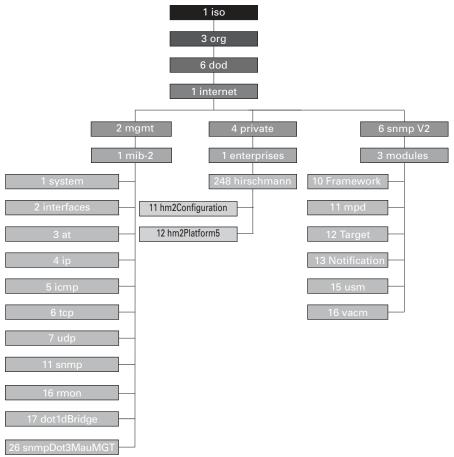
Figure 124: Tree structure of the Hirschmann MIB
