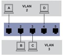
Figure 27: Example of a simple port-based VLAN
