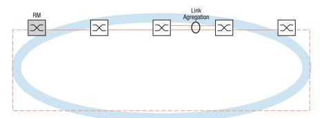
Figure 39: Link Aggregation over a single link of an MRP Ring.
