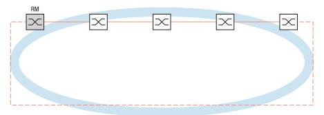
Figure 37: Redundant ring structure RM = Ring Manager — main line - - - redundant line
