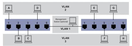
Figure 28: Example of a more complex VLAN configuration
