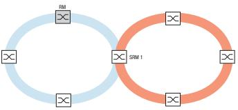
*Figure 54:* Special case: A Sub Ring Manager device manages both ends of a Sub Ring on different ports (Single Sub Ring Manger).
