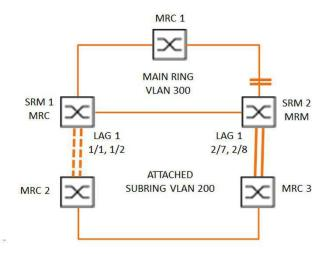
Figure 57: Sub Ring with Link Aggregation
