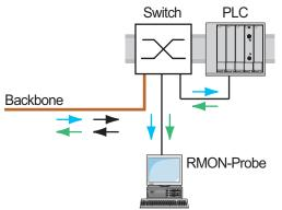
Figure 77: Application example of a port-mirroring setup
