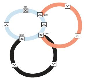
*Figure 53:* Special case: A Sub Ring Manager device manages 2 Sub Rings (2 instances). The Sub Ring Manager device is capable of managing up to 20 instances.
