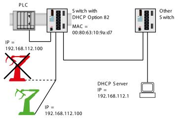
Figure 109: Application example of using Option 82
