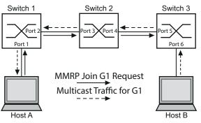
Figure 89: MMRP Network for MAC address Registration
