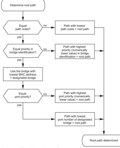
Figure 44: Flow diagram for specifying the root path
