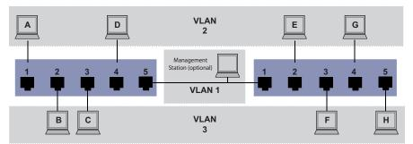
Figure 26: Example of a more complex VLAN configuration
