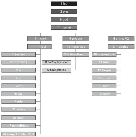
Figure 121: Tree structure of the Hirschmann MIB
