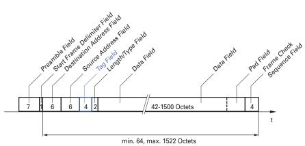
Figure 21: Ethernet data packet with tag
