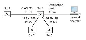
Figure 80: Application example of a VLAN mirroring setup
