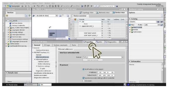
□ In the General tab, navigate to the *PROFINET* interface [X1] > Advanced options > Media redundancy item.
