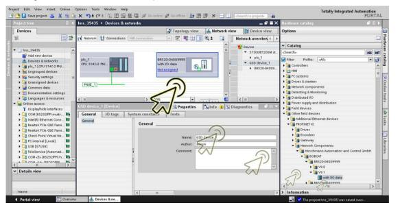
Assign the device to the PLC. To do this, click the *Not assigned* link in the device tile, then select the required item.
