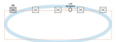
Figure 37: Link Aggregation over a single link of an MRP Ring.
