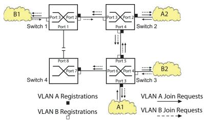
Figure 92: MVRP Example Network for VLAN Registration
