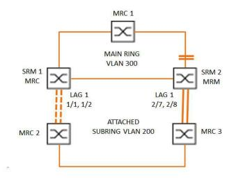
Figure 59: Sub Ring with Link Aggregation
