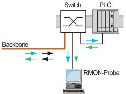
Figure 79: Application example of a port-mirroring setup
