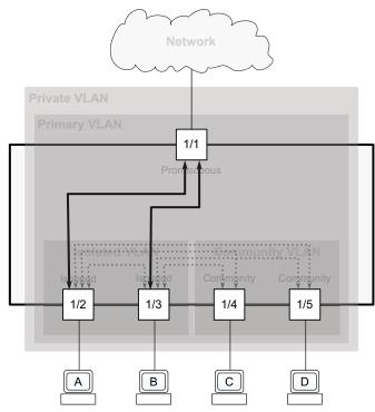
Figure 28: Communication flow of the isolated ports
