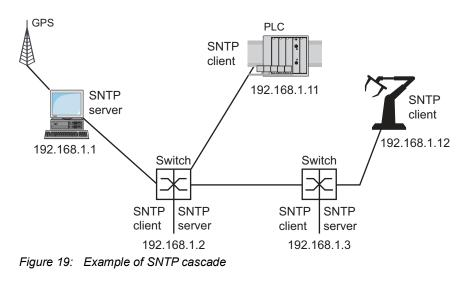
**Note:** For precise time distribution, between SNTP servers and SNTP clients you preferably use network components (routers and switches) that forward the SNTP packets with a low and uniform transmission time (latency).
