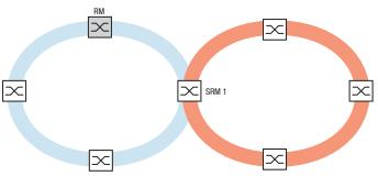
*Figure 56:* Special case: A Sub Ring Manager device manages both ends of a Sub Ring on different ports (Single Sub Ring Manger).
