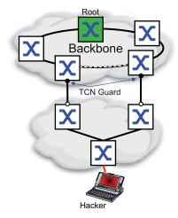
If the protection function is activated, then the device ignores *Topology Change* flags in received STP-BPDUs. This does not change the content of the MAC address table (forwarding database) of the device port. However, additional information in the BPDU that changes the topology is processed by the device.
