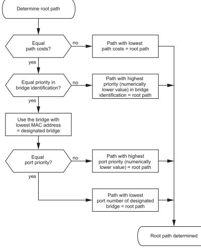
Figure 46: Flow diagram for specifying the root path
