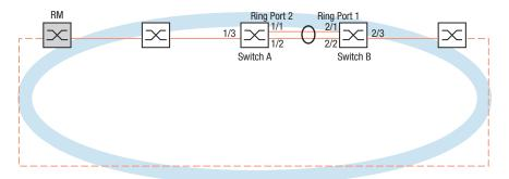
Figure 40: Application example of an MRP over LAG setup
