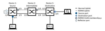
Figure 86: RSPAN in a line topology, using a reflector port (with separate uplinks)
