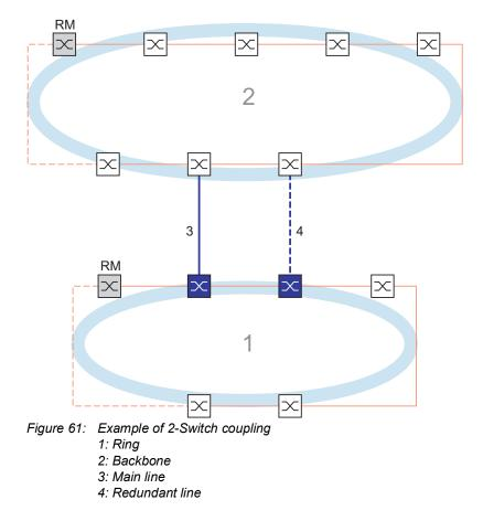
In a 2-Switch coupling (see figure 61), the 2 devices have specific roles:
