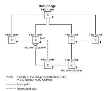
*Figure 49: Example of manipulating the tree structure*
