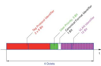
Figure 22: Structure of the VLAN tagging
