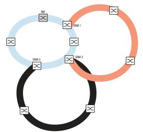
*Figure 55:* Special case: A Sub Ring Manager device manages 2 Sub Rings (2 instances). The Sub Ring Manager device is capable of managing up to 20 instances.
