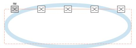
Figure 35: Redundant ring structure RM = Ring Manager — main line - - - redundant line
