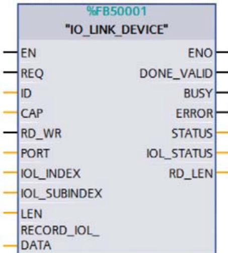
Abb. 32: "IO\_LINK\_DEVICE" FB in STEP 7 V15.1
