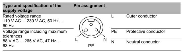
□ Connect the electrical wires to the socket according to the pin assignment.
