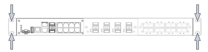
Figure 17: Mounting the MACH102 in the 19" cabinet
