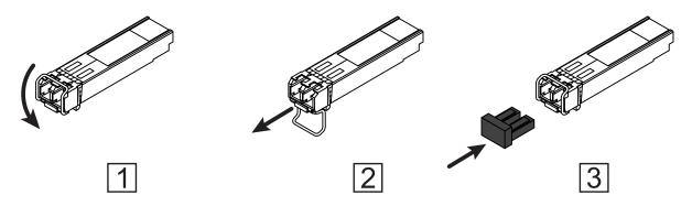
Figure 24: De-installing SFP transceivers: De-installation sequence
