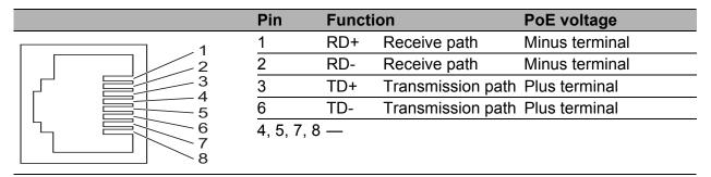
Table 7: Pin assignment 10/100-Mbit/s PoE port, RJ45 socket, MDI-X mode, phantom supply
