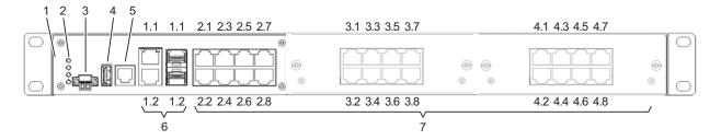
Figure 4: Overview over interfaces, display and operating elements of the MACH102-24TP-F, and MACH102-24TP-FR
