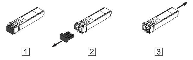
Figure 13: Installing SFP transceivers: Installation sequence
