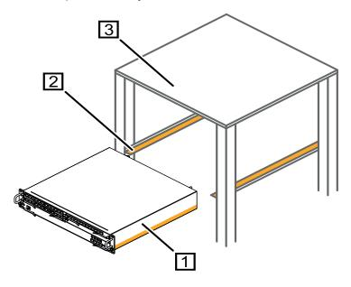
Figure 16: Assembly in a switch cabinet with sliding/mounting rails
