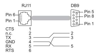
Figure 11: Pin assignment of the V24 interface
