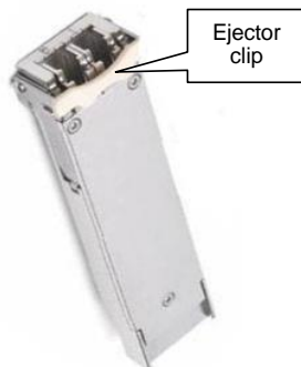
Optical XFP Module for PTN-1-10G-LW
