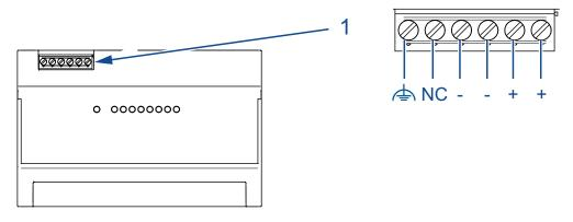
Figure 8: (1) Connection for DC voltage and AC voltage on the device
