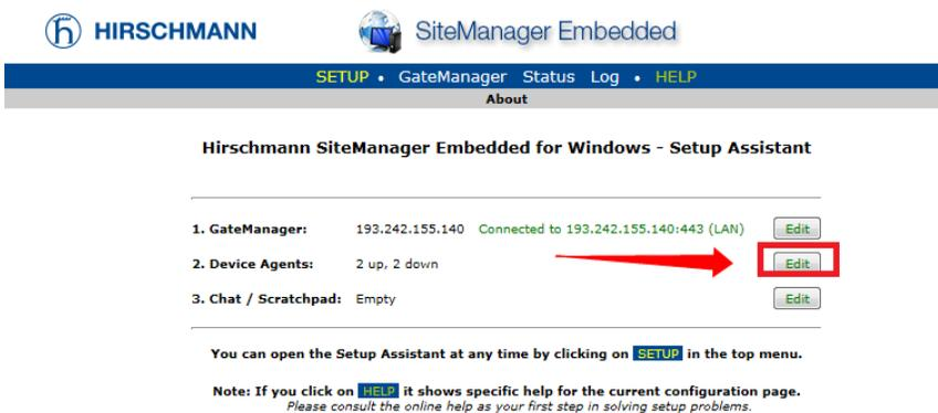
**Note:** The connection is made as a proxy connection via the GateManager, and is using a randomized port number, (in this case 55700 as indicated in the address line). Your outgoing firewall must support http and https access via the port range 55000-59999 for remote web access to work.
