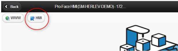
**NOTE:** The HMI button is only displayed if the agent can detect that the HMI server application is started.
