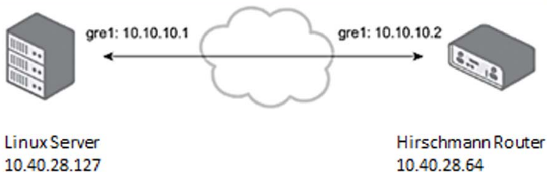
Figure 120: Example – GRE tunnel between Hirschmann router and OS Linux
