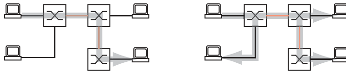
Figure 77: MAC Data Transmission: Unicast Data Packet (left) and Broadcast Data Packet (right)
