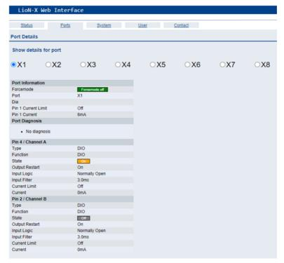
The page shows detailed port information. In the field **Port Diagnosis**, incoming and outgoing diagnostics are displayed as clear text. **Pin 2** and **Pin 4** contain information about the configuration and state of the port.
