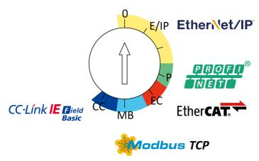
With the other rotary encoding switches (x10 / x1), you set the last two digits of the IP address when you are using EtherNet/IP, Modbus TCP or CC-Link IE Field Basic.
