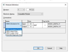
**12.** Select the connection type and configure the total sizes of the input and output process data. The sizes depend on the number of connected devices and their data lengths of both directions. Each device input and output data size must also be set later in the port configuration. The selection of the data type refers to the type in which Studio 5000® maps the input and output data. The default data type is SINT. The INT type is selectable when each size is
