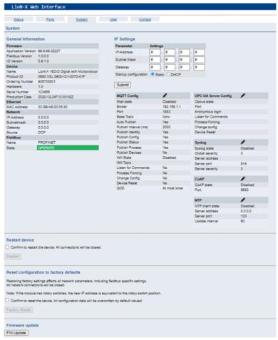
The System page shows the basic information for the module like Firmware version, Device information, Ethernet, Network and Fieldbus information.
