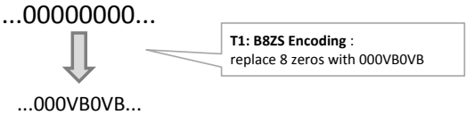
Figure 8 T1: B8ZS Encoding
