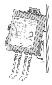
Fig. 8: Mounting a repeater on a DIN rail
