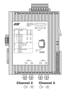
Fig. 10: Location of optical channels 2 and 3, with their respective inputs and outputs
