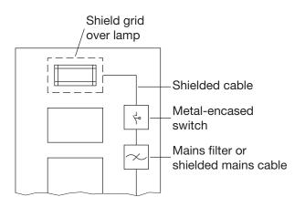
Fig. 5: Interference suppression of fluorescent lamps in cabinet
