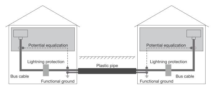
Fig. 7: Laying cables outside of buildings
