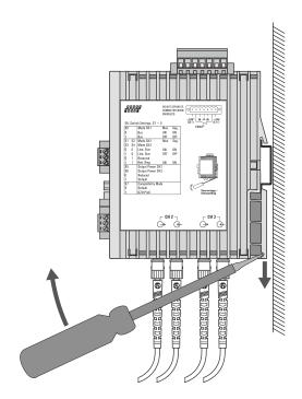
Fig. 9: Removing the repeater from a DIN rail
