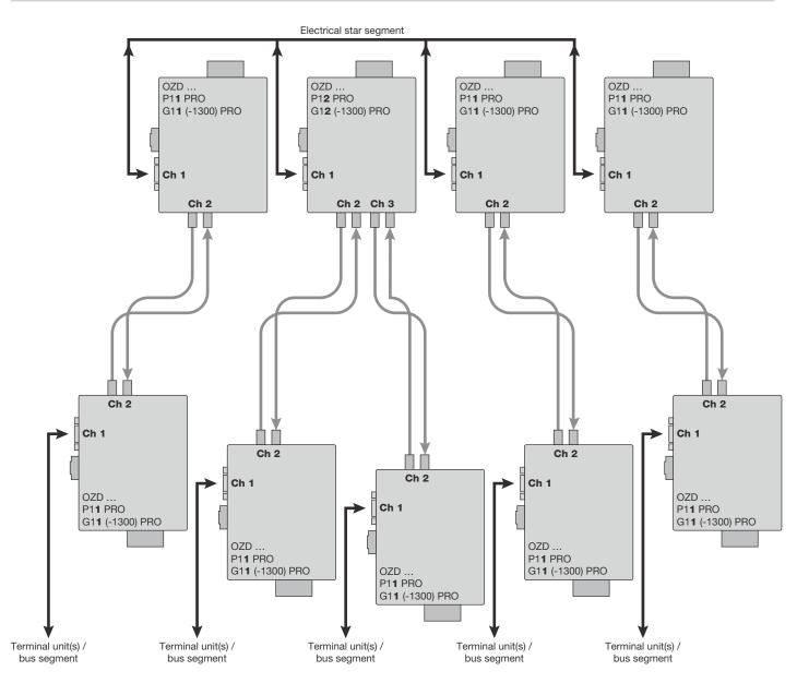
Fig. 4: Network structure in an optic star topology
