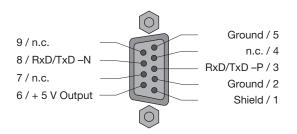
Fig. 11: Electrical channel – assignment of Sub-D socket
