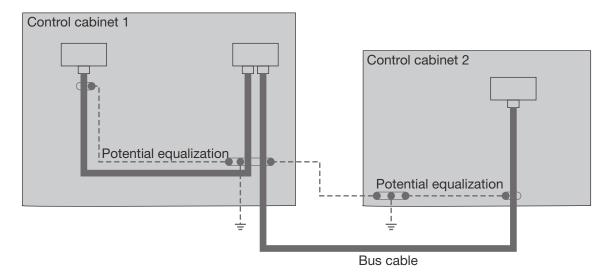
Fig. 6: Laying cables inside of buildings
