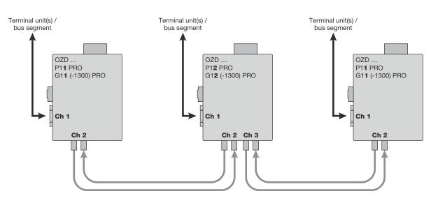
Fig. 2: Network structure in an optical line topology
