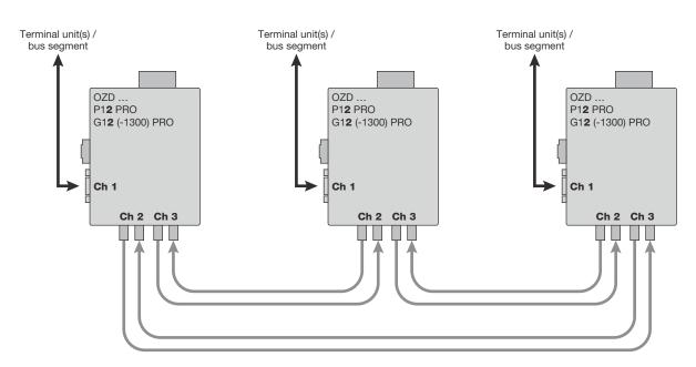
Fig. 3: Network structure in a redundant optical ring topology
