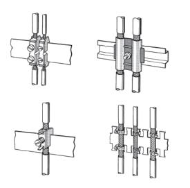
Fig. 6: Securing shielded lines using cable clamps and tube clips (schematic diagram)
