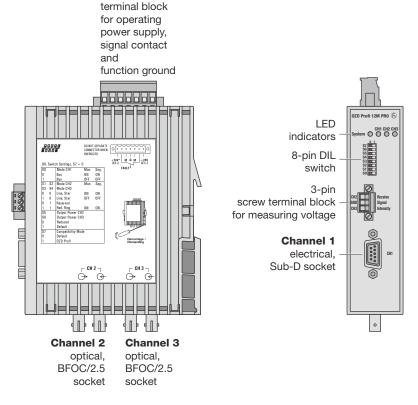
Fig. 1: OZD Profi 12M ... PRO repeater showing the location of the LED indicators, measuring sockets and the individual channels.
